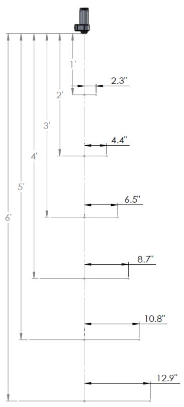
Figure 1: Vehicle Clearance versus Height Above Surface
